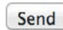
Figure 10.13 A submit button created by way of the <input> element with a type attribute value of submit
