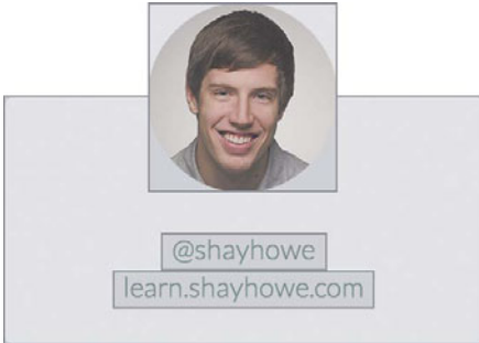
Figure 4.2 When we look at each element individually, we can see how they are all rectangular, regardless of their presented shapes
