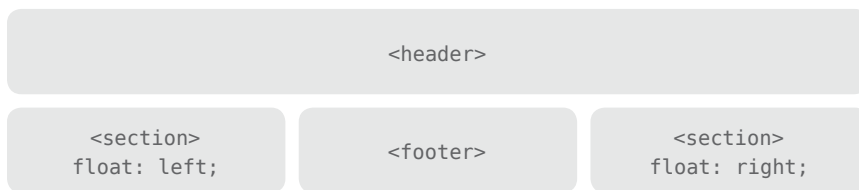
Figure 5.4 A two-column page layout without any identified column widths or cleared floats
