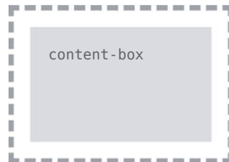
Figure 7.15 The content-box value contains the background within the border and padding of an element
